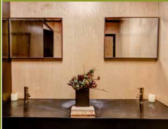
In the women's powder room, Lujan and Blea repeated many of the materials used throughout the restaurant: Maple walls are offset against a hand-cast black concrete sink with an "invisible drain" underneath a small maple screen; the brass faucets reference the brass rivets used throughout the main restaurant room. The duo also fabricated the wall and door to the toilet area (on left) out of blackened steel.
